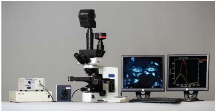
FIGURE 1. The HSI microscope system includes a smooth spectrum halogen light source, spectral imager (Headwall Photonics), color camera (Dage-MTI, Michigan City, IN) and automated stage (Prior Scientific). Dual monitors allow the image and spectral data to appear on separate screens.
