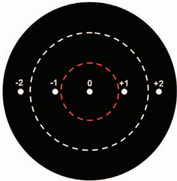
Figure 2 Diffraction pattern produced by a simple object and impact of NA. Red ring: small collecting angle of a low-NA objective (e.g., 0.10), white ring: collecting angle of a moderate-NA objective (e.g., 0.44), full aperture: collecting angle of a larger-NA objective (e.g., 1.3 oil immersion).
