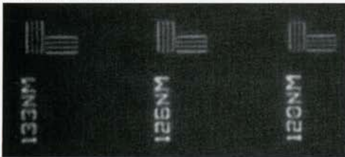
Figure 1. This portion of the Richardson Test Slide offers a series of parallel vertical and horizontal lines with distances between lines of 133, 126, and 120 nm. The last resolved pattern would indicate the horizontal and vertical resolution of a microscope. Olympus BX51, CytoViva150, 100X, oil, NA1.4, color digital camera, Sony DXC-S500.
