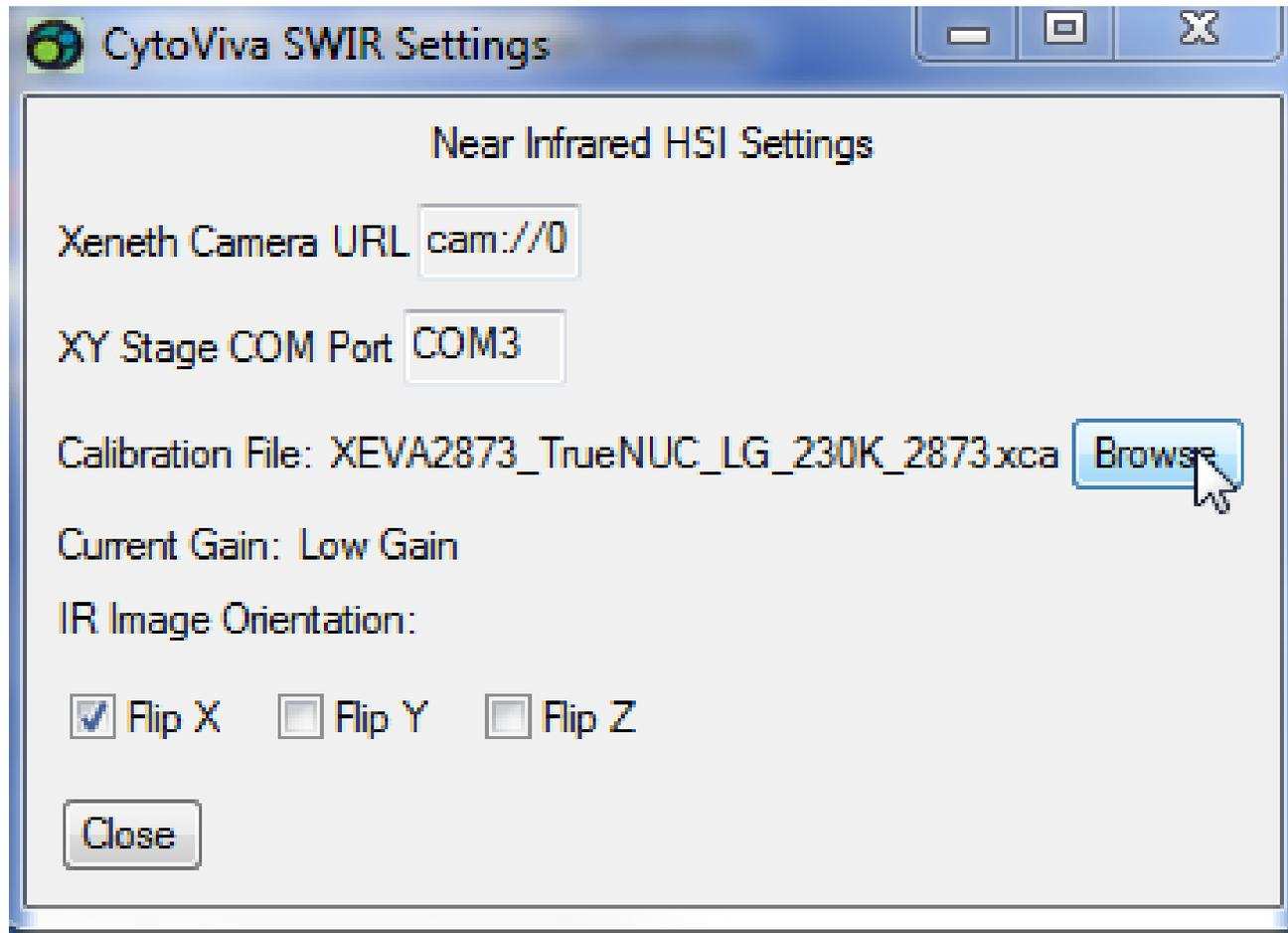
5. Navigate to the folders in the image below and select the XEVA file that says “1S-HG”. This file will allow exposures for up to 1 second and operate the camera in High Gain mode. Once this file is selected it will always be the default file. This “1S-HG” file is made specifically for CytoViva so Elyse will make sure it is on the same USB stick that comes with the camera. You can copy it into this directory so it is easy to find. Once its in this folder it should stay there.
