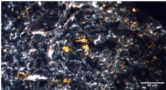
Figure 3: Au Nanoparticles (Areas Observed as Gold) Aggregating in Tissue 60x
