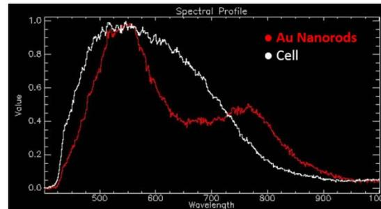
Figure 2: Spectral Response of Au Nanorods (red) and Cells (white)
