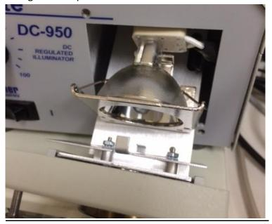
3. Slide the bulb out of its holder between the metal plate and 2 retaining clips.
