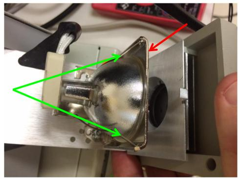
7. Push lamp housing back up against main body and tighten both screws.
