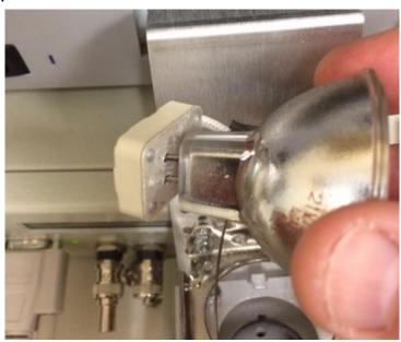
5. Place the new bulb in the socket and make sure the 2 prongs are all the way in the ceramic plug.
