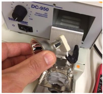
6. Place the bulb back in its housing sliding it between the metal plate and the 2 retaining clips.
