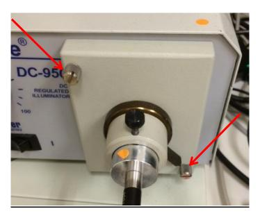
2. Pull the lamp housing out to expose the socket that connects to the bulb.
