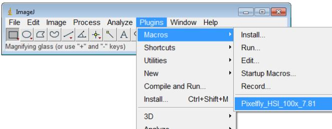
e) After selecting the macro, you will be presented with the image with the scale bar added. Make sure to save the file before closing as the files with the added scale bar is not automatically saved
