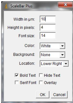
f) After selecting OK, you will be presented with the image with the scale bar added. Make sure to save the file before closing as the files with the added scale bar is not automatically saved
