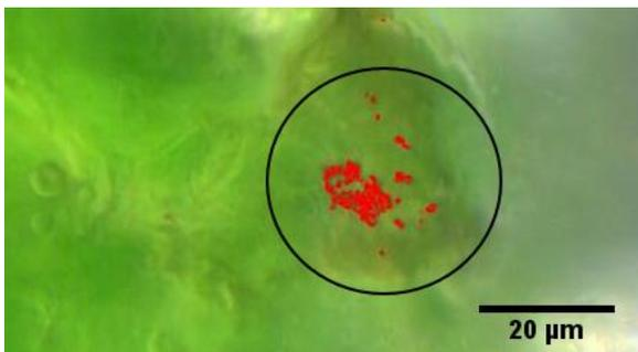
Figure 2: 60x Enhanced Darkfield Hyperspectral Image with Selenium Mapped and Pseudo-Colored Red
