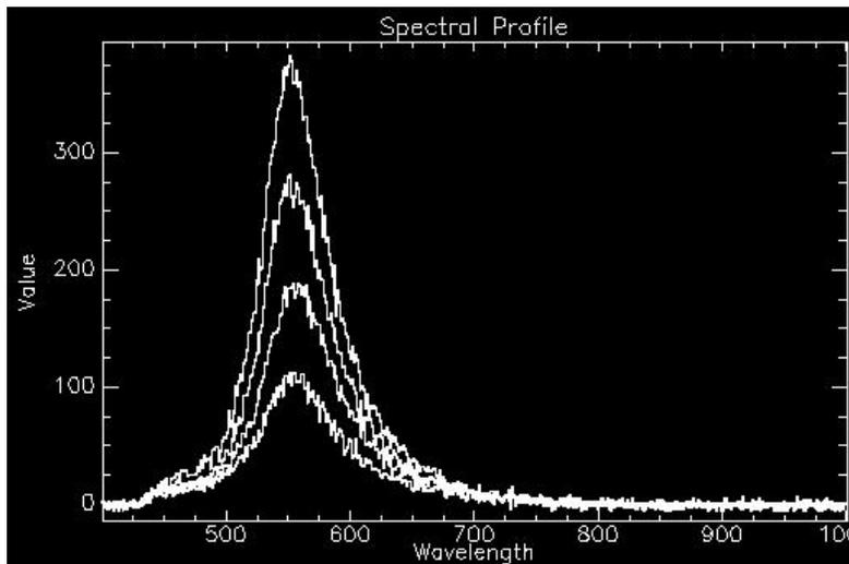
Figure 6: Time Resolved Spectral Changes of a Single AuNP Measured at 200 Milliseconds with Reduced Output of the Source Illumination Decreasing the Nanoparticle Peak Amplitude
