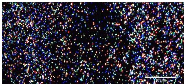
Figure 1: 30nm AgNPs Aggregating in DI Water
