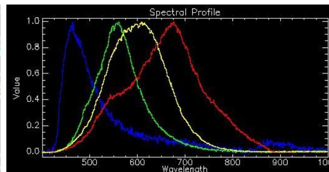
Figure 2: Spectral Measurements of Aggregating AgNPs in DI Water
