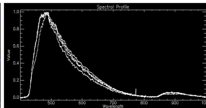
Figure 4: Spectral Measurements of Dispersed AgNPs in an Ionic Solution
