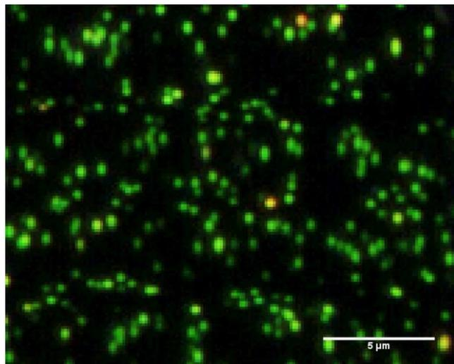
Figure 5: Enhanced Darkfield Hyperspectral Image of 50nm AuNPs at 100x Plus 4x Digital Zoom
