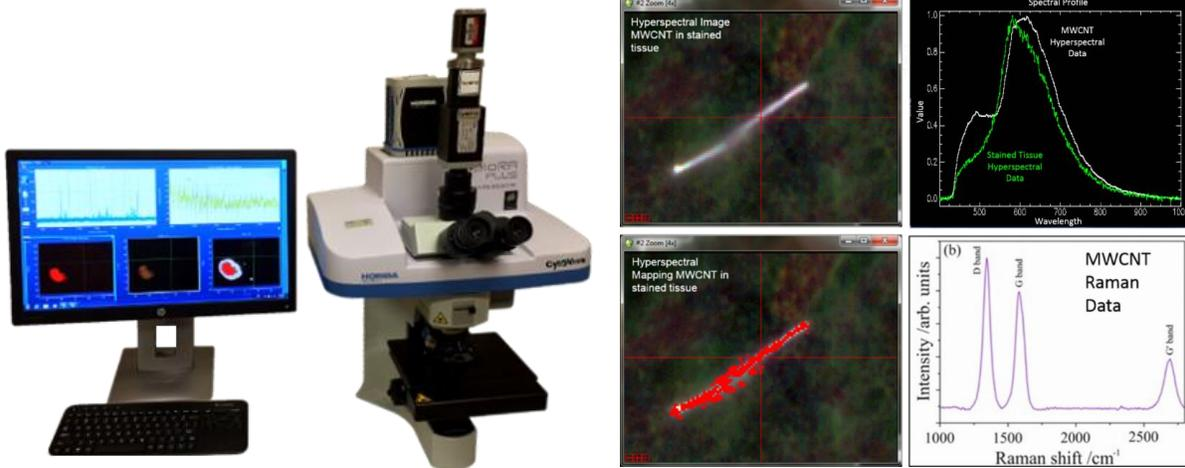
In collaboration with HORIBA Scientific, CytoViva now provides confocal Raman imaging integrated on the same microscope platform as its enhanced darkfield and hyperspectral imaging system. This integrated solution meets a critical need for nanotechnology researchers in that it combines the benefit of high spatial and spectral resolution, enhanced darkfield hyperspectral imaging and the quantitative molecular analysis provided by Raman.
