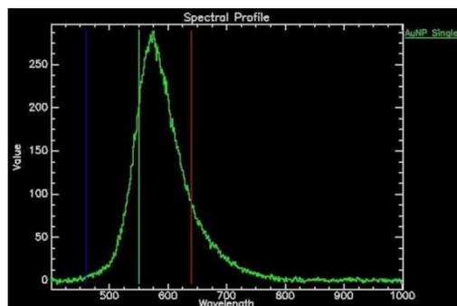
Figure 4: Plasmon resonance based spectral response of the AuNPs.
