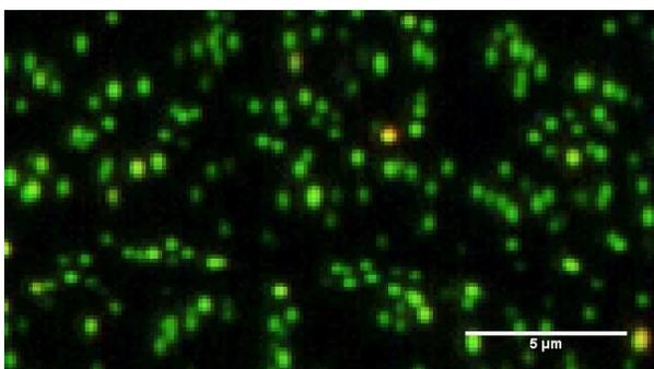
Figure 3: 50nm AuNPs on a glass slide.
