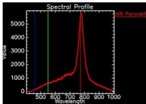
Figure 2: Emission spectrum of Perovskite nanocrystal area circled red in figure 1.
